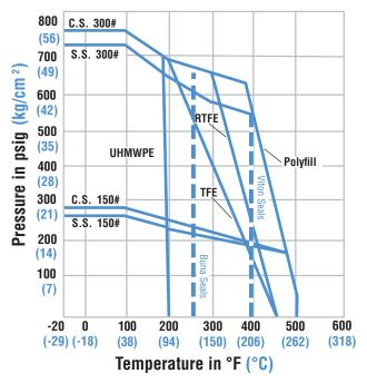
NOTE: Maximum working pressure limited by both flange rating and seat capability.
